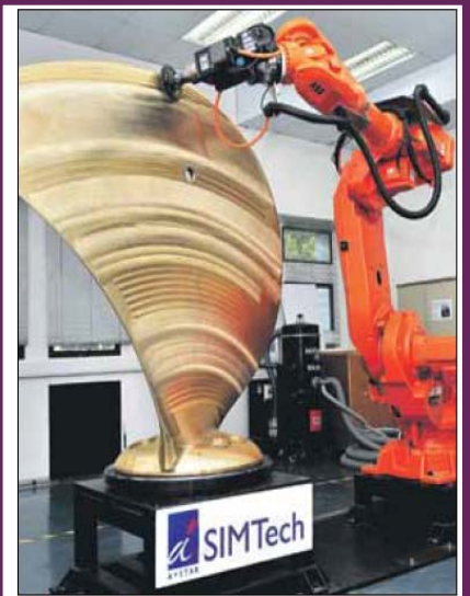
A demonstration of how a robotics system is used to polish the surface of a marine propeller. PHOTO: A*STAR
